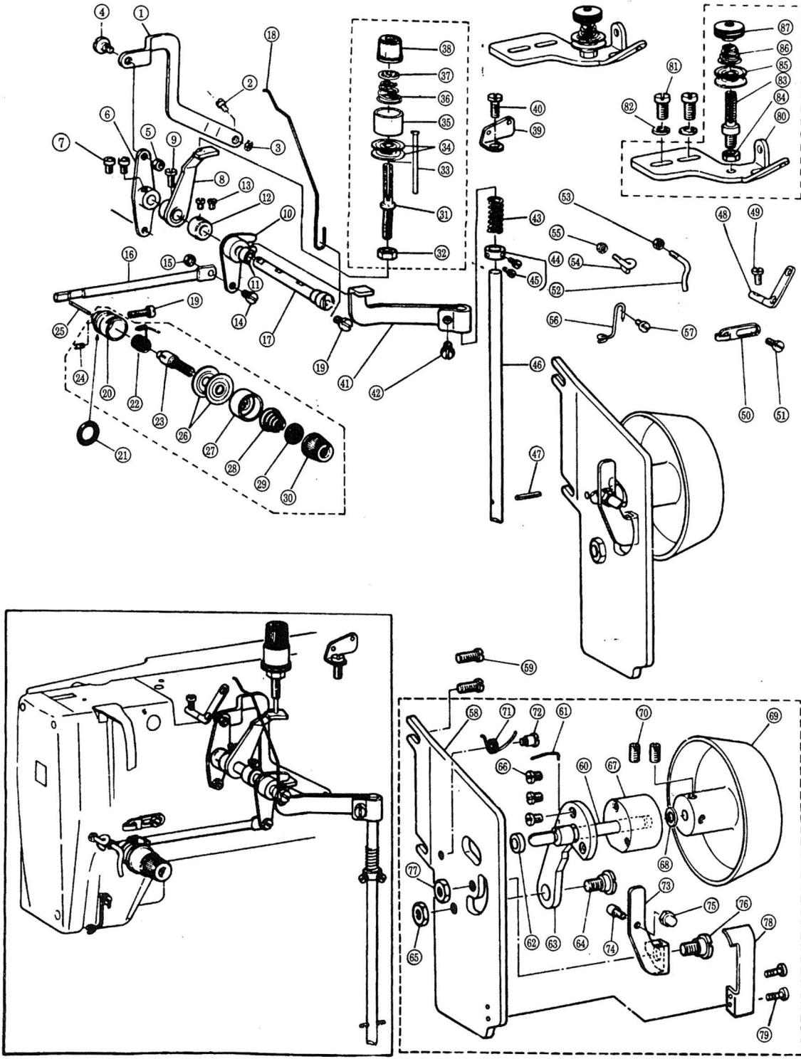
**14、润滑系统分组件****14.Lubrication mechanism components**
