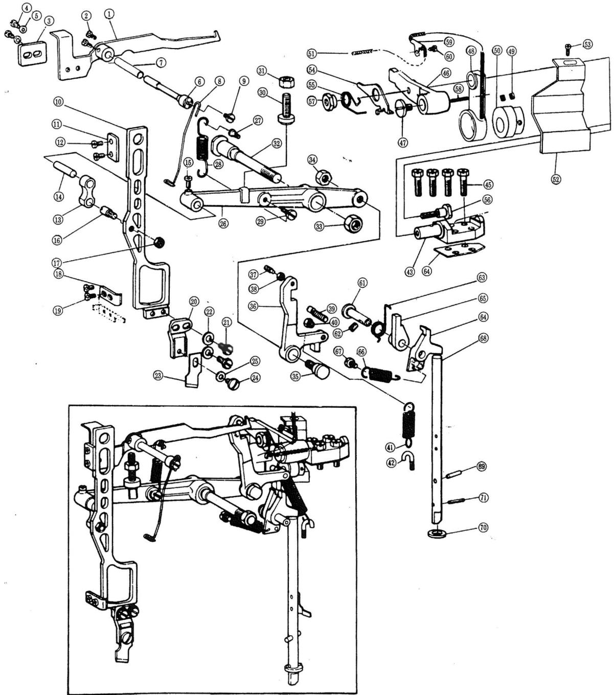
**10. 送料凸轮分组件****10. Feed cam and tripping Segment Components**
